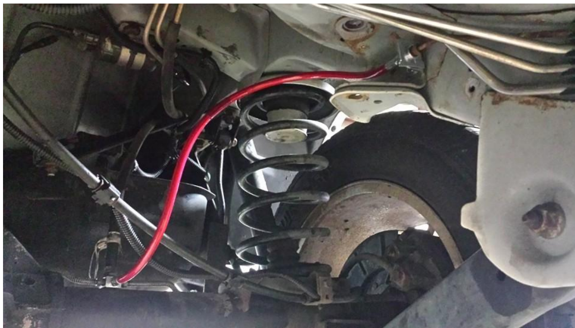
Rear brake line with distribution block at axle and frame-end fitting
