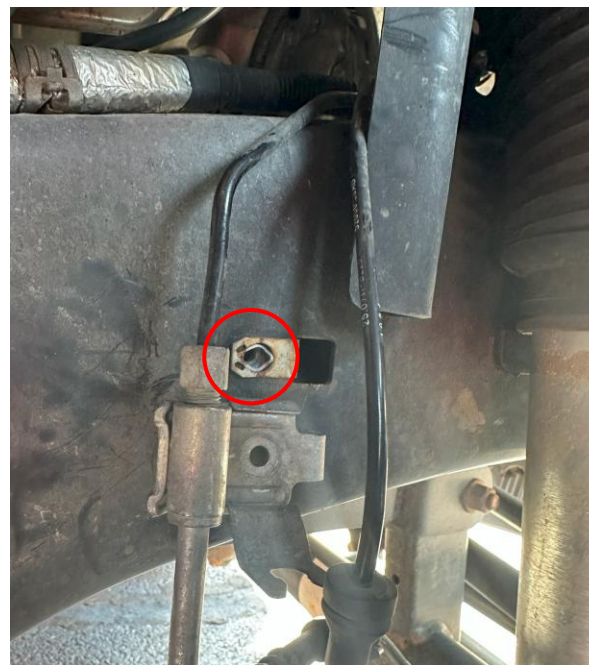
Frame bracket before and after removal (10mm)
