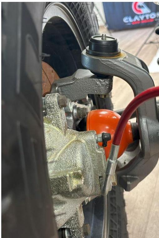
banjo fitting installed (front driver's side)
