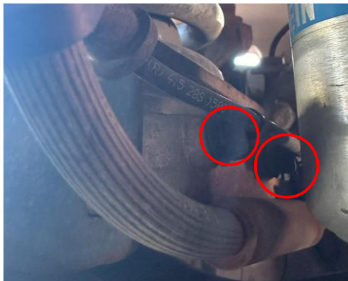
Coil bucket zip ties to be cut
