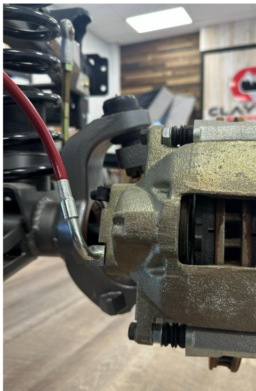
OEM front brake line orientation
