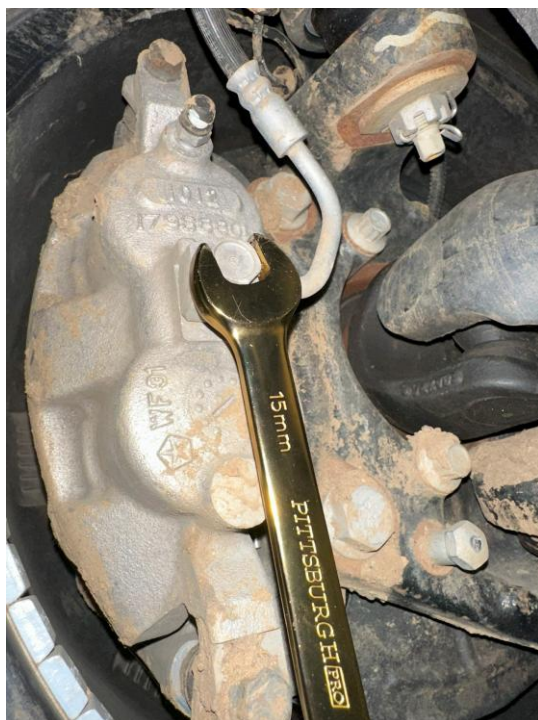
Brake caliper banjo bolt (15mm)
