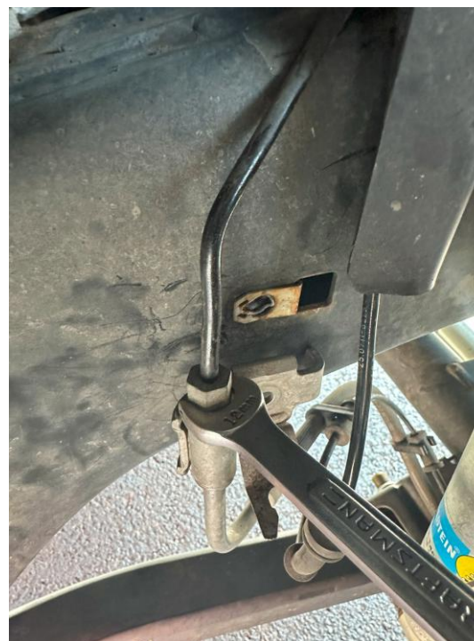
Frame end fitting (12mm)
