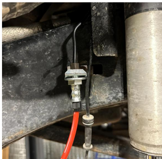
Brake line mounting process
