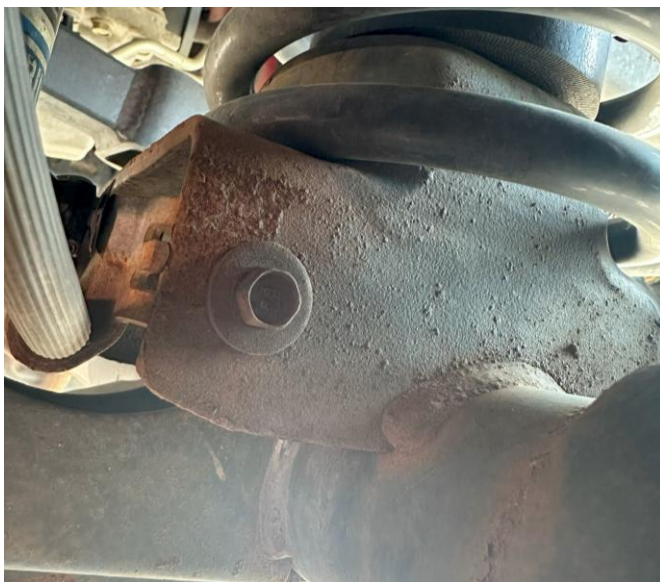
Coil bucket brake line bracket bolt to be removed (10mm)
