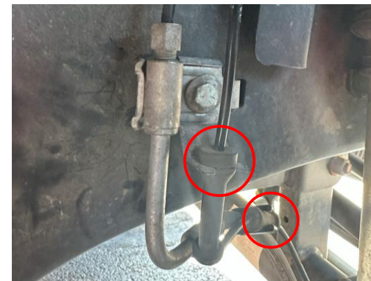
Frame mount ABS cable to be removed
