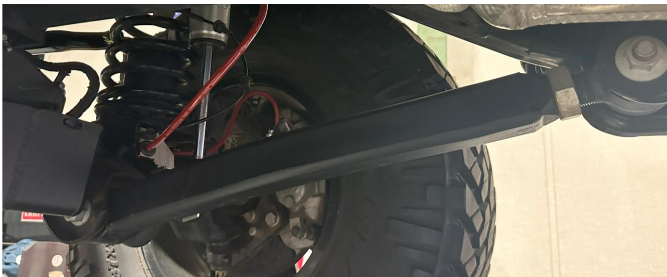
1708100 (OVERLAND+ Series) Front lower control arm installed on Jeep JT
