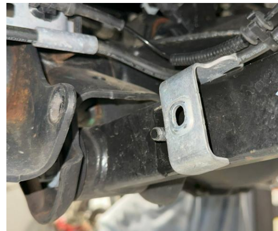
Brake line bracket removed on driver side
