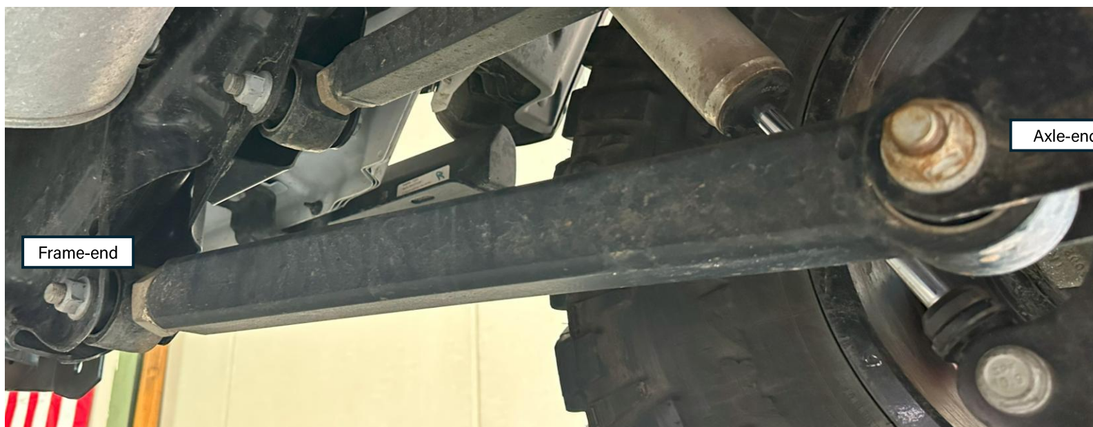
1710102 (OVERLAND+ Series) Rear lower control arm installed, passenger-side (Jeep JT)
