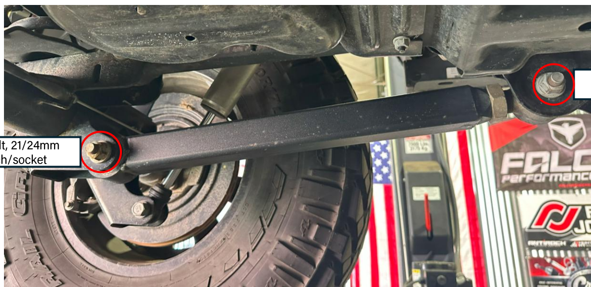
1710102 (OVERLAND+ Series) Rear lower control arm installed (frame-end and axle-end)
