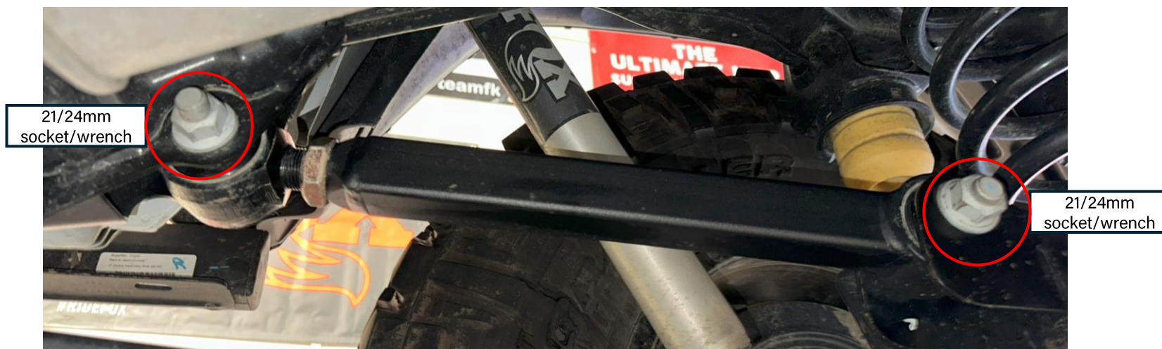
1710103 (OVERLAND+ Series) Rear upper control arm installed
