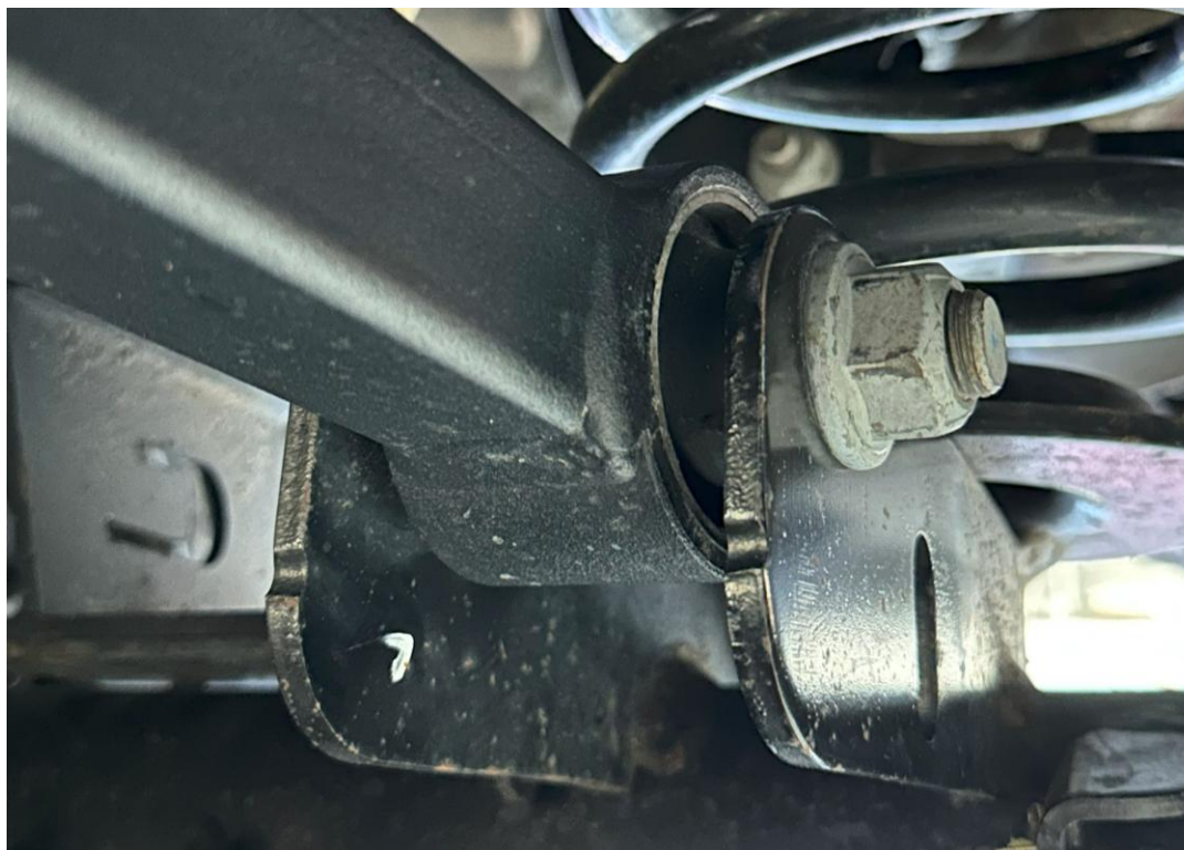
1710103 (OVERLAND+ Series) Rear upper control arm installed, axle-end
