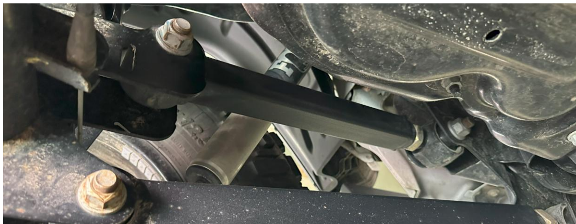
1710103 (OVERLAND+ Series) Rear upper control arm installed
