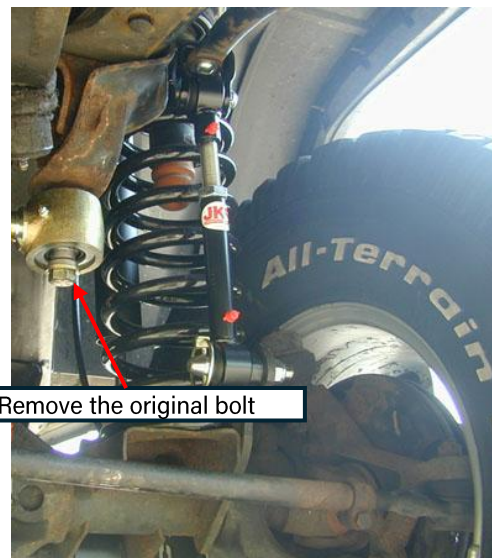
XJ frame-end track bar mount (bolt to be removed)
