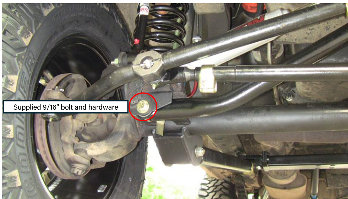
XJ axle mount track bar fully installed
