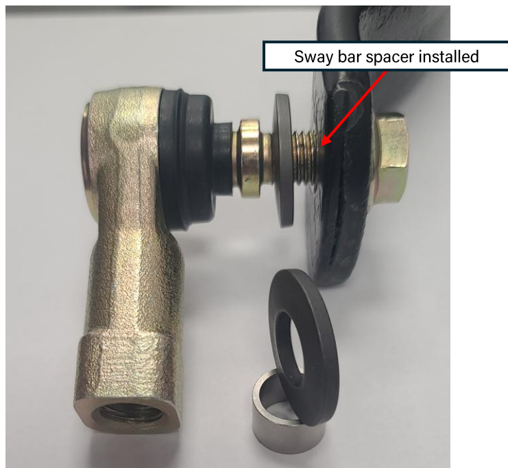
Figure 2: Sway bar bushing spacer installed inside sway bar
