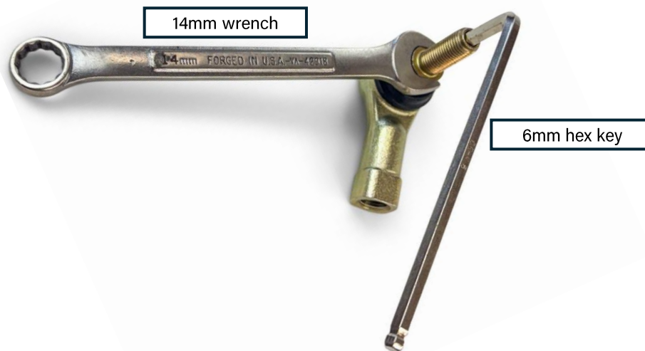
Figure 7: Rod end tightening options
