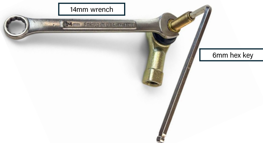
Figure 5: Rod end tightening options
