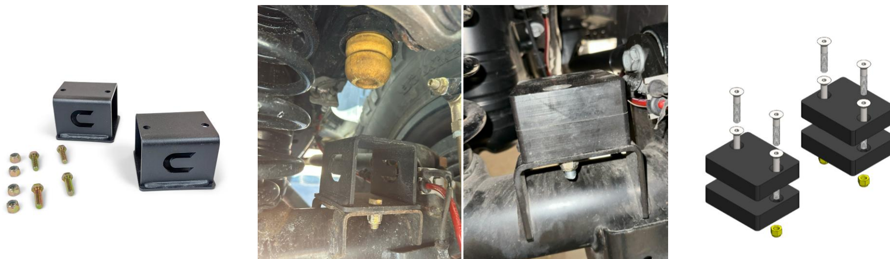
Figure 33: Bump-stops (3" tall and 1-2" tall stackable bump-stop options)
