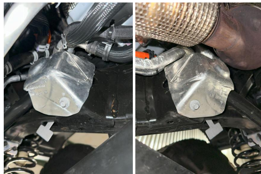
Figure 7: Front upper control arm heat shields to be removed
