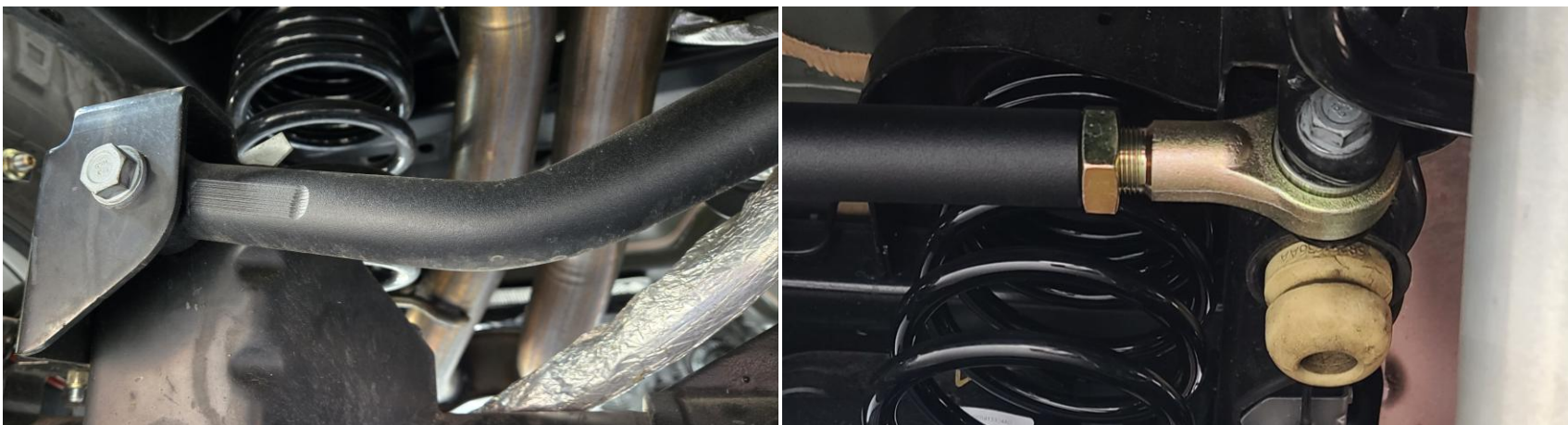
Figure 32: New rear track bar installed
