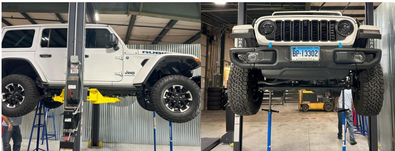
Figure 1: Vehicle supported by lift and jack stands
