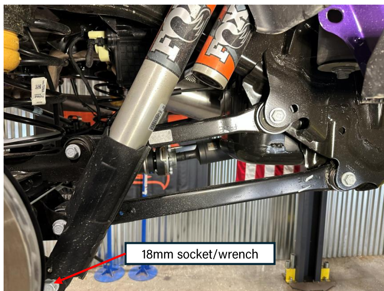
Figure 21: Rear passenger/driver-side lower shock bolts to be removed
