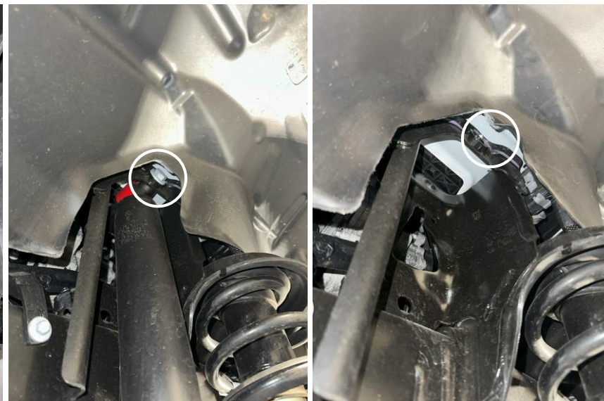
Figure 5: Front upper passenger shock bolt removed
