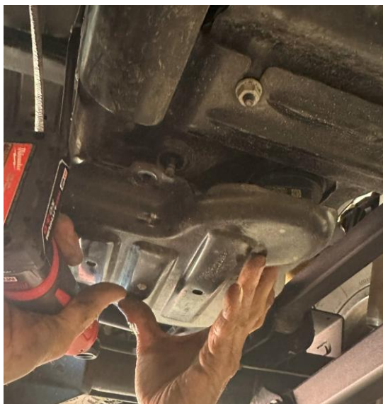
Figure 33: Removing x3 nuts at bottom plate
