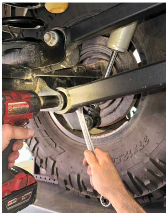
Figure 51: Removing rear lower short arm
