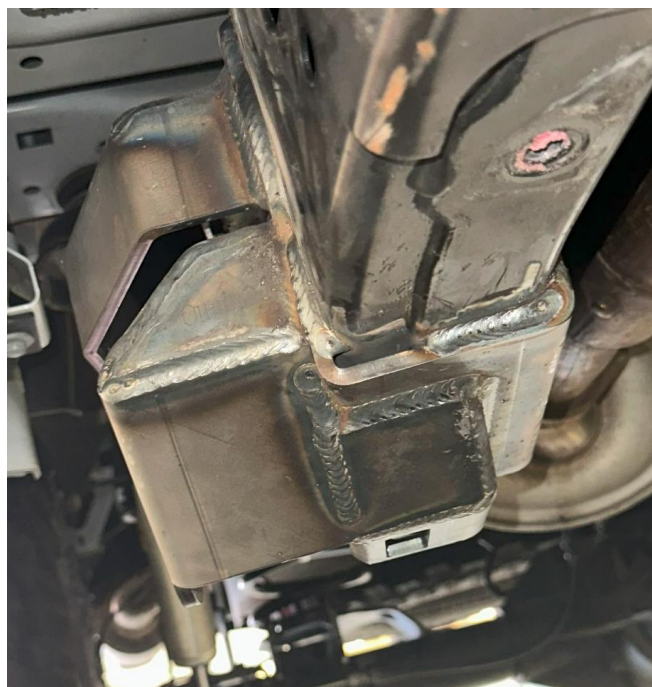
Figure 48: Rear of bracket welds
