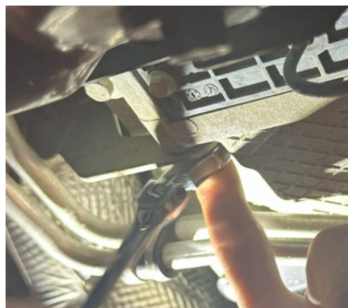
Figure 4f: Front hanger removal
