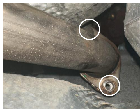
Figure 4c: Flange to be removed (x2 bolts)
