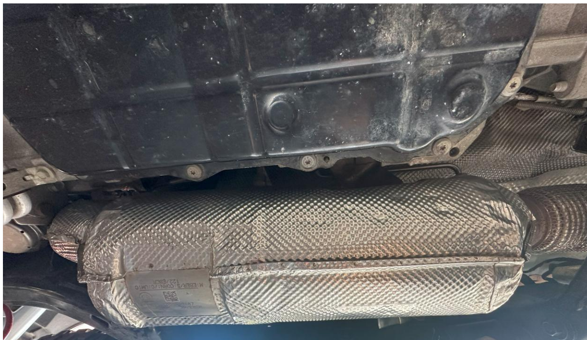
Figure 57: Catalytic converter reinstalled under the vehicle
